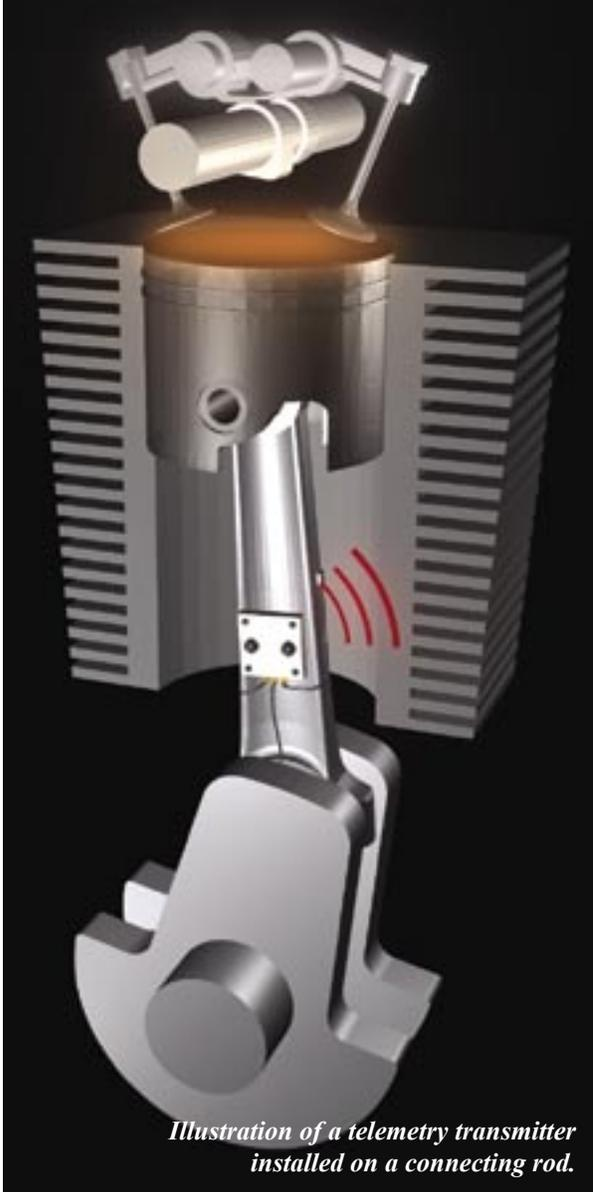
*Illustration of a telemetry transmitter installed on a connecting rod.*
