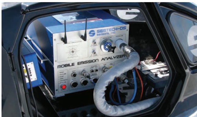
Mobile emissions analysis system collects emissions and fuel consumption data while the vehicle is "in-use."
