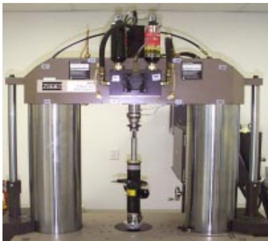
Figure 1: MTS 831 Machine with Shock Absorber Installed
