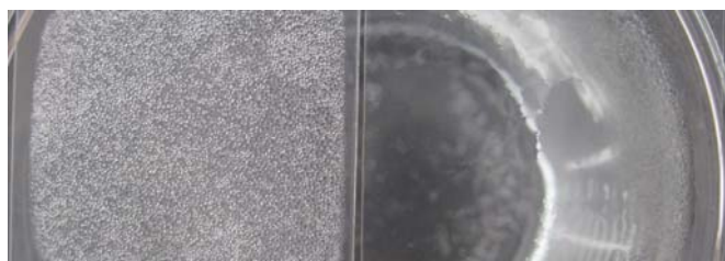
Fig. 2. Condensation and optical clarity of polyester films under high relative humidity. Left side: untreated polyester film is fogged. Right side: plasma-treated superhydrophilic polyester film keeps optical clarity.
