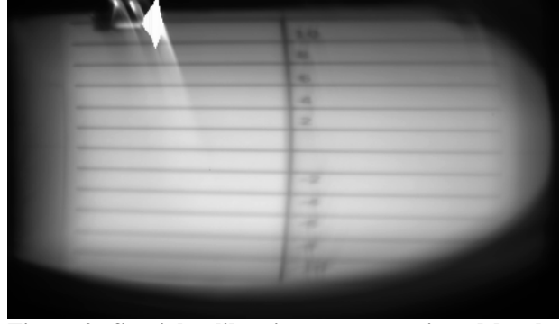
Figure 2. Spatial calibration target as viewed by the spectrograph
